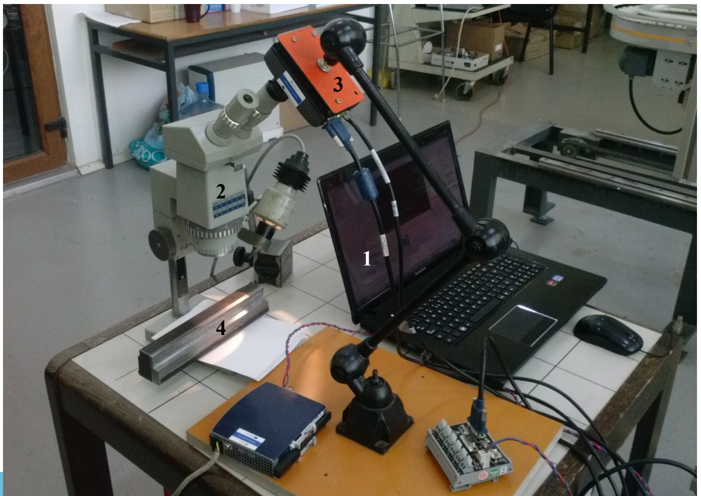
Figure 3. Image acquisition stand (1 – Laptop, 2- optical microscope,
